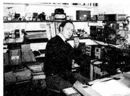
Dave Jones, GW3SSY, secretary of Abergavenny & Nevill Hall ARC, is seen at the controls of his station. The rigs are, l to r, a Heathkit HW9, HW101, Yaesu FT480R, and FRG7700
